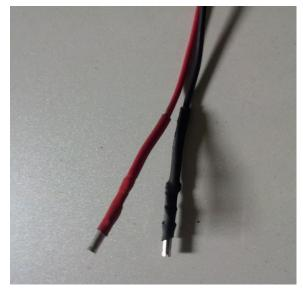
Looking at the light with the bolt on the left side. The pin on the left is ground and the pin on the right is positive. The positive wire should be hooked up to a wire that activates when you press the brake light.
