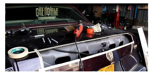
*Tip: Use a flat earth magnet to keep the bracket in place while you are test fitting and making adjustments. These are available on eBay and they come in handy when doing custom body work. Also note the spacing of the bracket in this picture, the cut out should be as close to the bracket as possible.*
